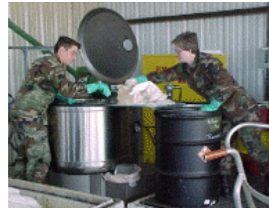
Loading JP-8 soaked absorbents into the industrial centrifuge
